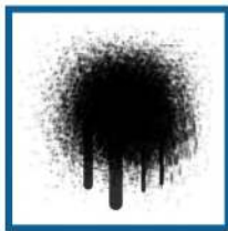
Too much paint produces these drippings
