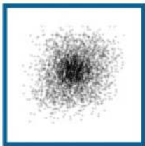
Too much air flow produce this splatters
